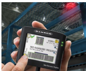
RD35 Handheld Remote Display Used for- programming
