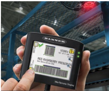
RD35 Handheld Remote Display Used for programming
