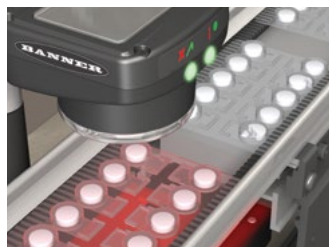
Area Sensor — Detects whether a particular feature (features) are present
